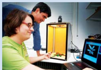
VOLKER LANNERT/JUNI BONN Researchers Tim Wigbels (L) and Julio Pastrana test their weed recognition software and leaf-blasting laser system.
