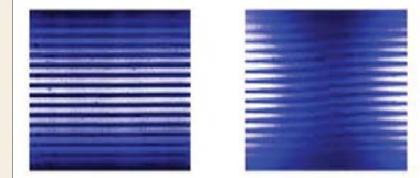
UV radiation from a relativistic electron beam is diffracted by a double-slit. In contrast to the normal light (L), the diffraction shows a deformation in the central part (R), indicating the existence of the phase singularity, which is a definite evidence of the vortex nature.
