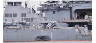
The damaged port aft hull of USS John S. McCain, left, is seen while docked next to USS America at Singapore's Changi naval base on Tuesday, Aug. 22, 2017 in Singapore.
