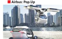
Best known for its double-decker A380 jet, Airbus premiered its solution for urban transit at Geneva international motor show in March. The Pop.Up consists of a carbon-fibre passenger capsule that functions as a two-seater electric car when attached to a chassis, or as an aircraft when a drone is summoned by smartphone to remove the capsule from the chassis.
