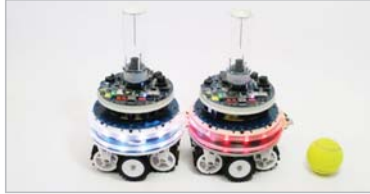
These Roomba-like robots latch onto each other with metal clasps and merge their 'nervous systems' to become bigger, centrally controlled bots of various shapes and sizes.
