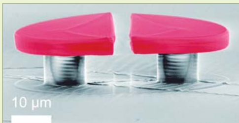
phys.org Scanning electron micrograph of a polymeric WGM split-disk cavity: Two opposing half-disks ( R=25\mu\text{m} ) with an intermediate air gap of several microns are structured onto an elastomeric PDMS substrate with direct laser writing.
